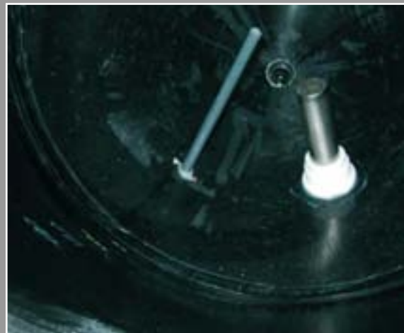
Fig. 84 - Internal view of tanks in Fig. 83: the heater and the thermostat probe
